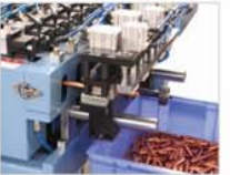
刀头旋转，无屑切割 cutter-rotating ,chipless cut
